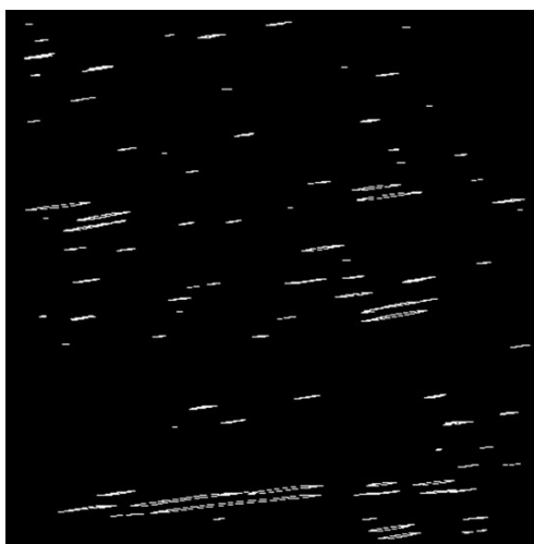
Fig. 6 Extended lines in Fig. 5 were identified by convolving with a linear segment of the appropriate orientation, thresholding to find regions of a large enough length, and dilating to correct for end effects.
